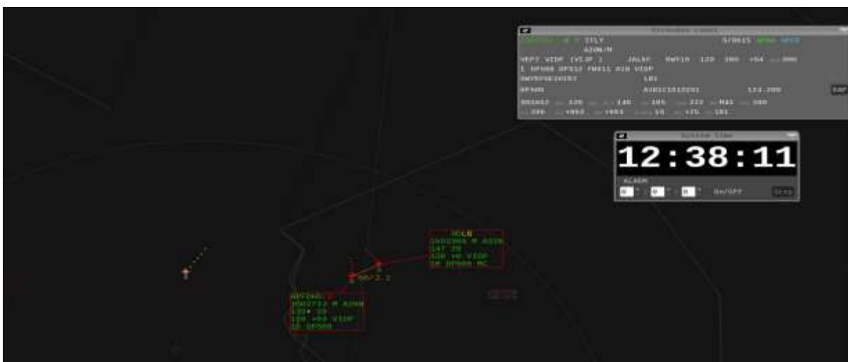
Fig 6: Current Conflict Alert appeared at 12:38:11 UTC
