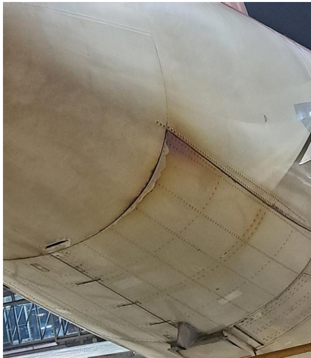
APU compartment (in fuselage tail cone) and access doors on the bottom of the tail cone [Post incident]
