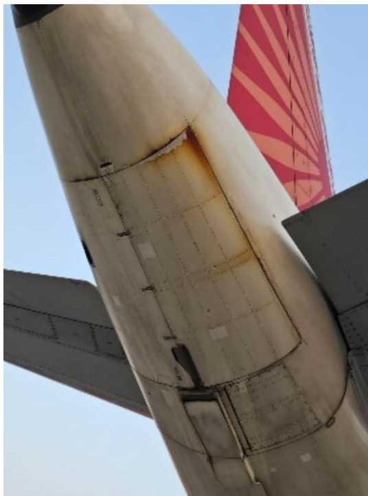
APU compartment (in fuselage tail cone) and access doors on the bottom of the tail cone [Post incident]
