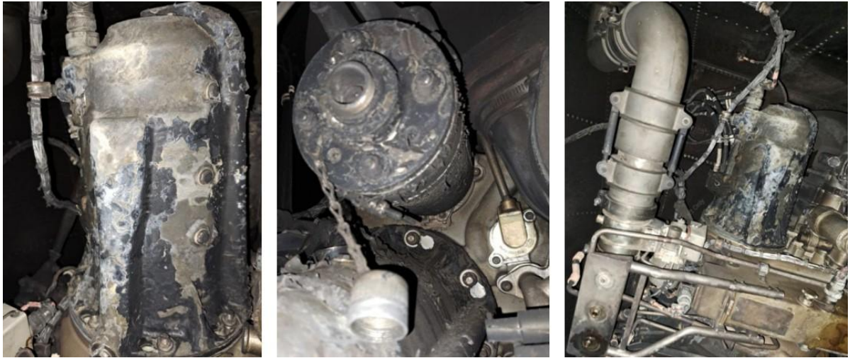
2. Traces of oil found on oil tank, oil LOP Switch and APU Drain Port
