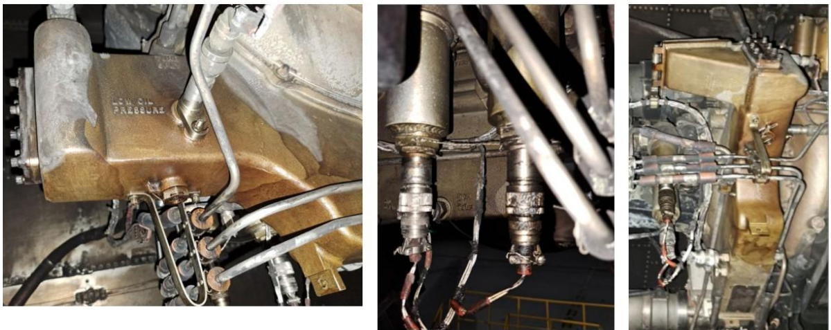
2. Traces of oil found on oil tank, oil LOP Switch and APU Drain Port
