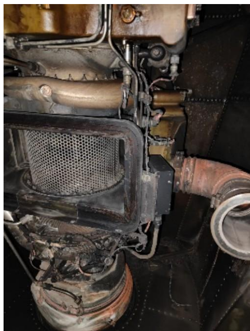
APU compartment (in fuselage tail cone) and access doors on the bottom of the tail cone [Post incident]
