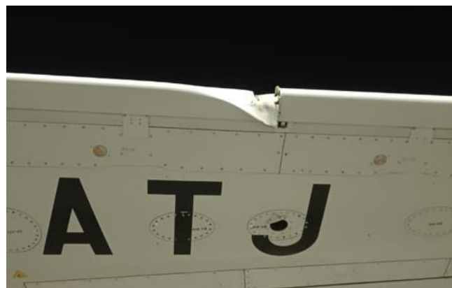
Fig.3: Damage to Slat#5 of LH wing
