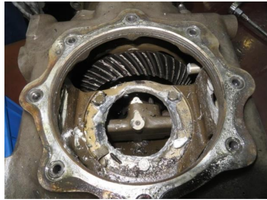
Figure 20: TGB housing excessive damage and wear
