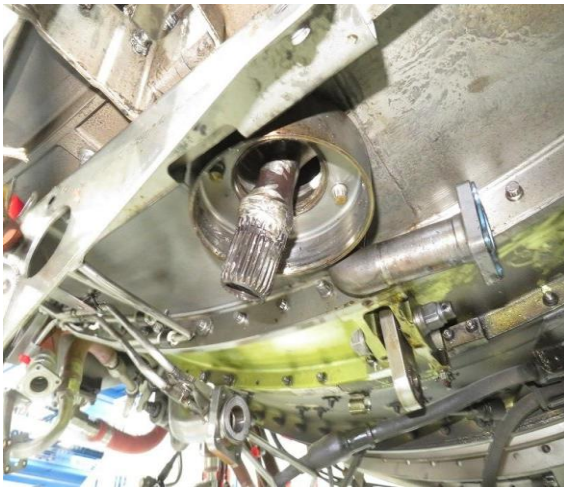
Figure 13: Outer housing broken and wear
