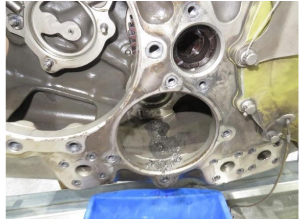
Figure 26: Large amount debris in AGB lower area
