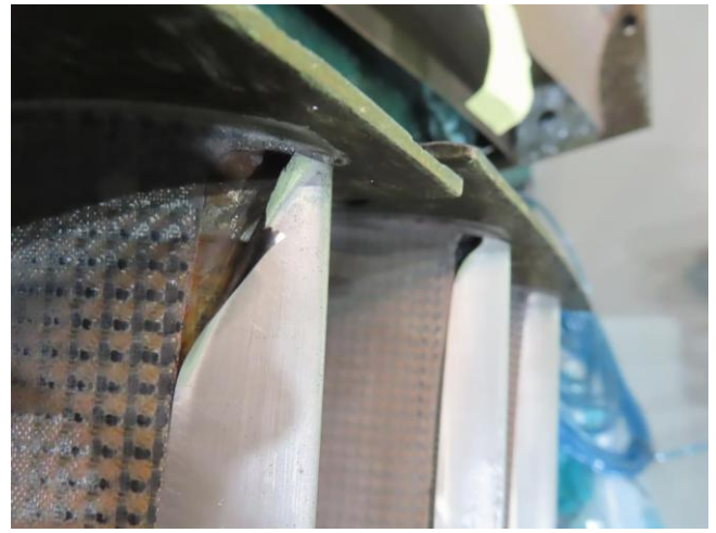
Figure 14: OGV Leading edge metal sheet un-bond
