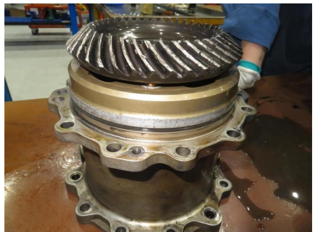
Figure 24: Output gear damage
