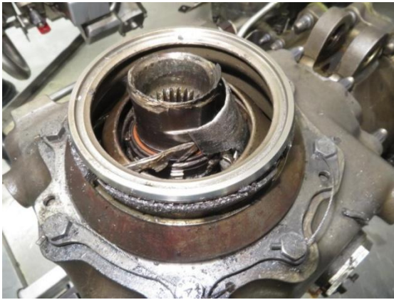
Figure 19: TGB input adapter security bolt with wrong safety
