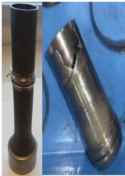
Figure 27: Comparison of RDS inner housing upper side remaining section with good condition
