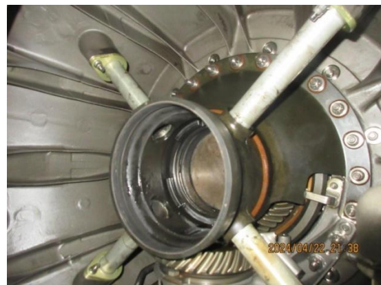
Figure 18: FWD oil stationary seal seized with IGB
