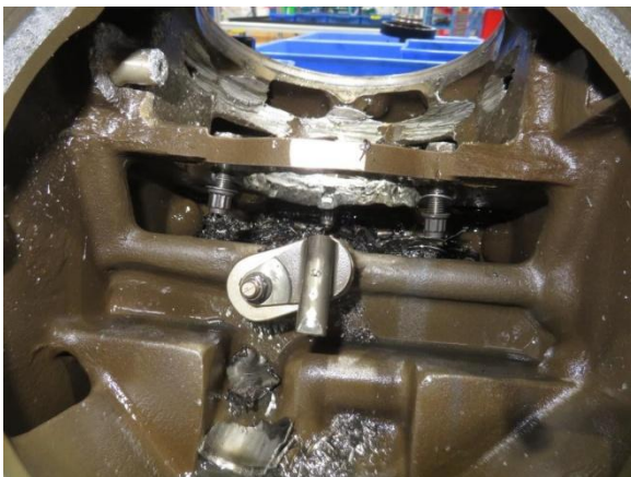
Figure 21: TGB housing excessive damage and wear
