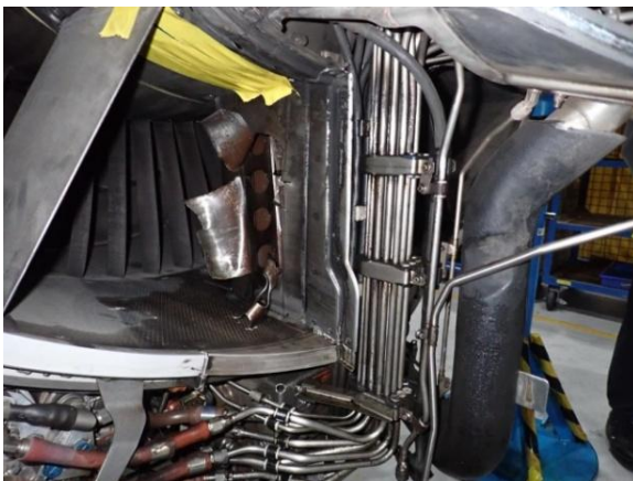
Figure 11: Fan frame strut 7 significant damage
