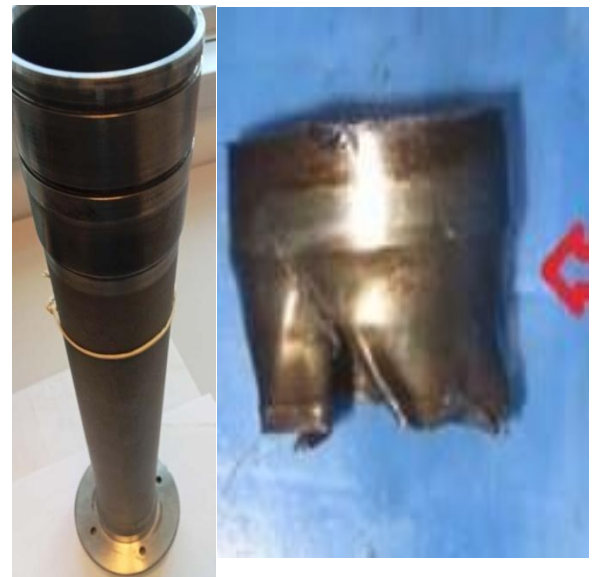
Figure 28: Comparison of RDS outer housing upper side remaining section with good condition
