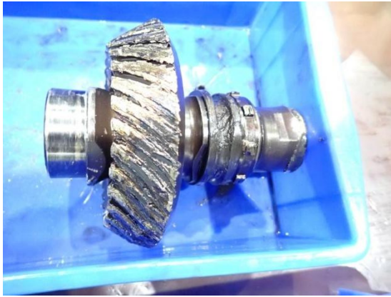
Figure 25: TGB input shaft excessive damage
