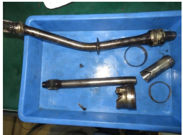
Figure 22: RDS shaft broken
