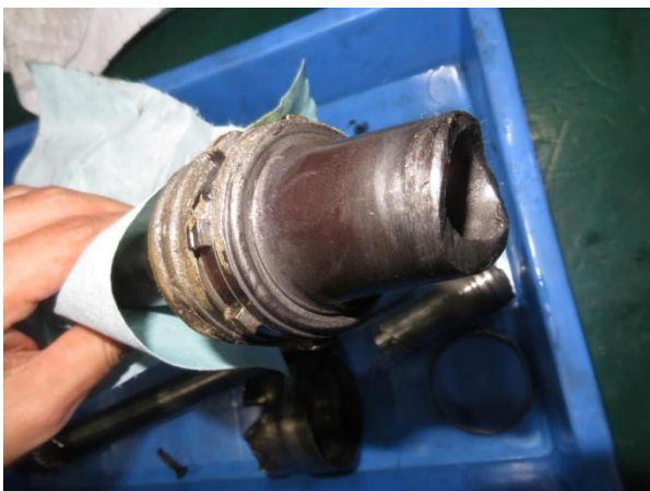
Figure 23: RDS Bearing missing
