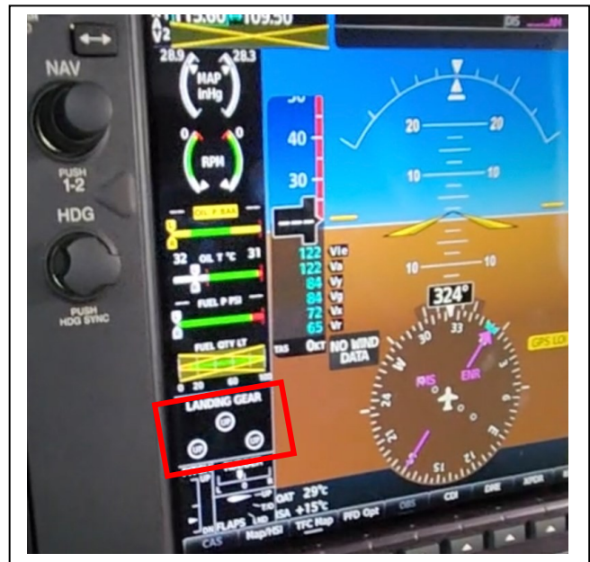
Fig. 5: Landing gear uplock showing on the PFD
