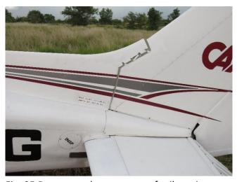
Fig. 05 Damage to bottom part of tail section
