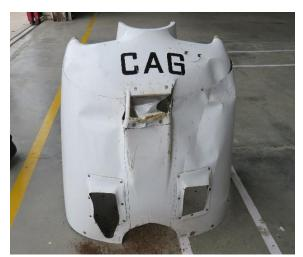
Fig. 06 Damage to the bottom cowling
