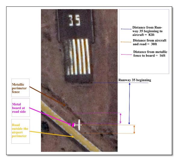
Fig.12. Aircraft position after coming to halt-aerial representation (not to scale)
