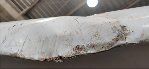
Fig. 02 Damage to the port side wing leading edge
