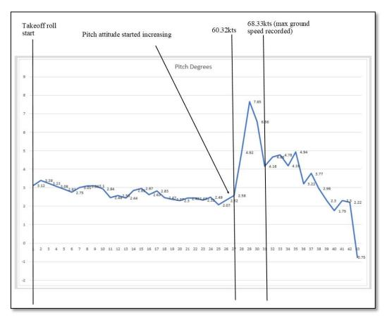
Fig.08 Pitch degree vs relevant time
