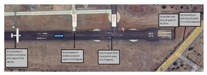
Fig.09 Aircraft ground speed and pitch correlation
