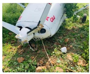
Fig. 04 Propeller damage
