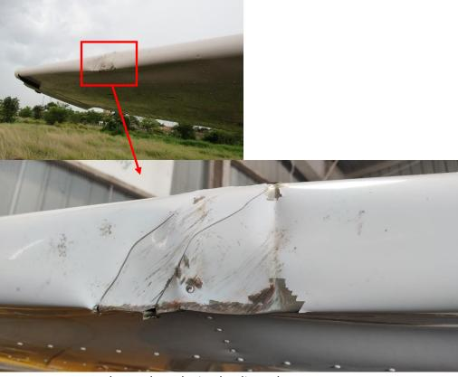
Fig. 01 Damage to the starboard wing leading edge
